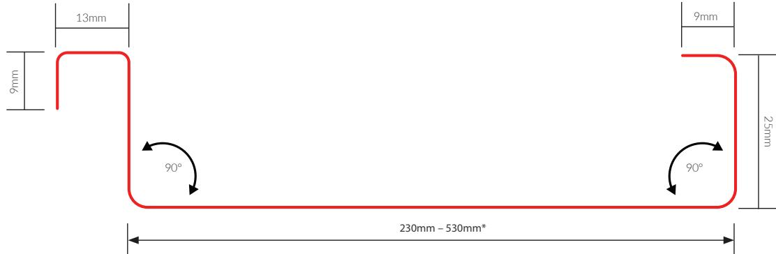
Non-combustible metal cladding and roofing profile
