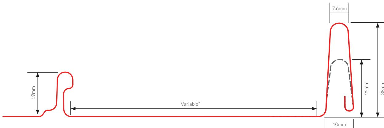
Non-combustible metal cladding and roofing profile, our recommendation is for Striplok to be used as wall cladding only
